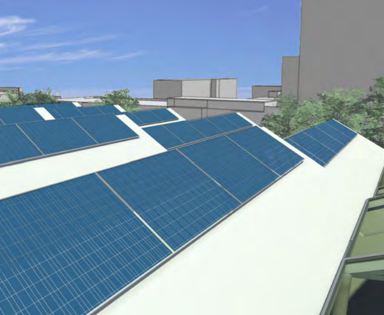
4.5. ROOF DESIGN WINDOWS ON THE NORTHERN ROOFS / PHOTOVOLTAIC PANELS ON THE SOUTHERN ROOFS OF BUILDING A
