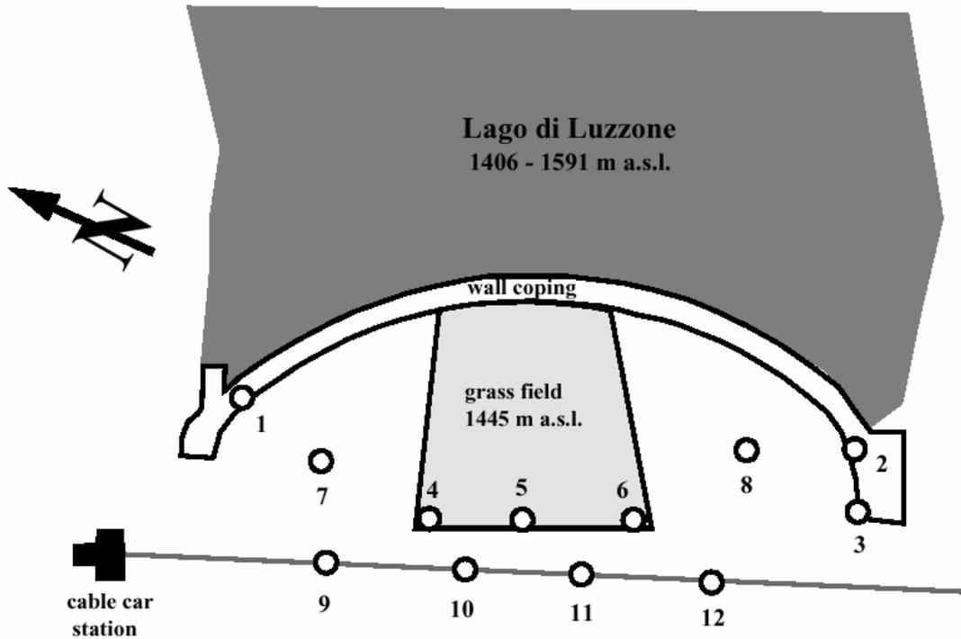
Figure 5: Configuration of camera stations for DCS200 at dam Luzzone
