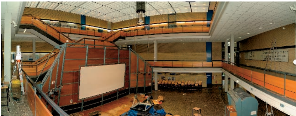
Fig. 2: 3D test field at the Hafencity University Hamburg for geometrical investigations into TLS systems.
