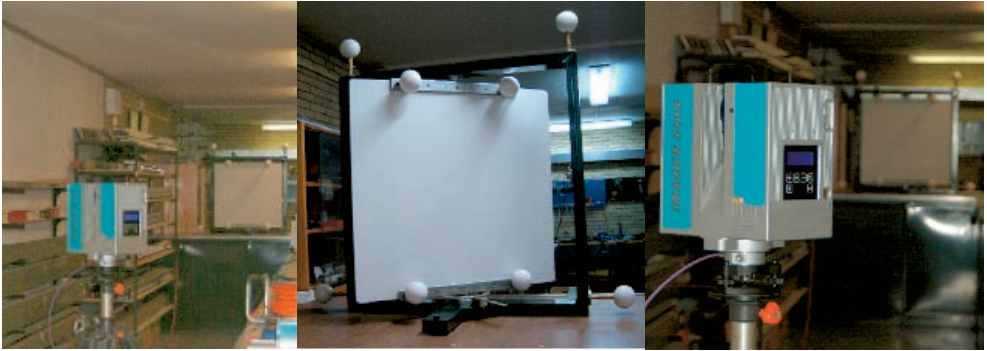
Fig. 11: Scanning set up for the investigations into the laser beams angle of incidence on 3D accuracy with swivelling planar white stone slab (centre).
