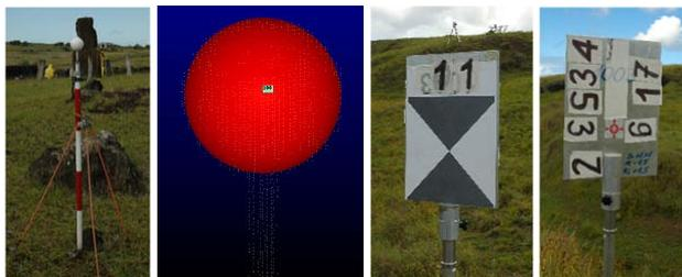
**Fig. 2:** From left to right: Marked point with white sphere for registration and geo-referencing of scans from GX/GS101, scanned and recognised sphere for GS101, front side of the target for IMAGER 5006 and back side of the same target for geodetic point determination and a flexible numbering system.
