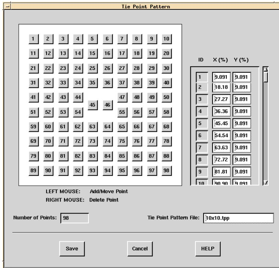
Figure 2: Tie point pattern used for automatic tie point extraction in the OEEPE/ISPRS test data
