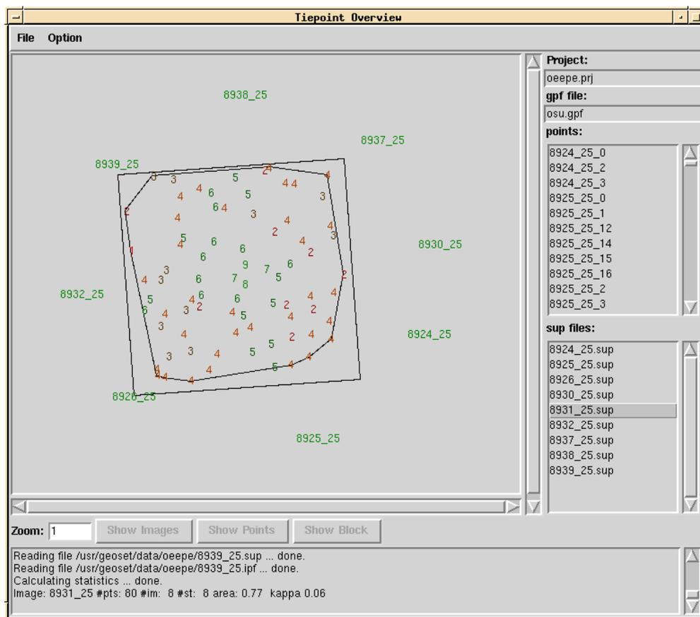
Figure 3: Visualisation of photo connections within a triangulation block for quality control
