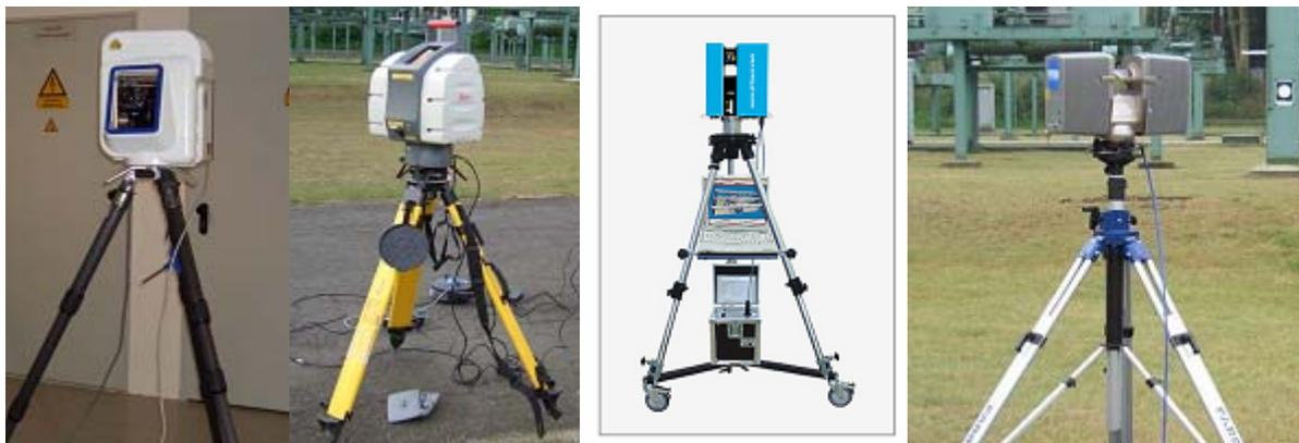
Fig. 1: The used terrestrial laser scanning systems for the comparison tests: Trimble GS101, Leica Scan-Station, IMAGER 5003 from Zoller & Fröhlich, Faro LS 880HE.
