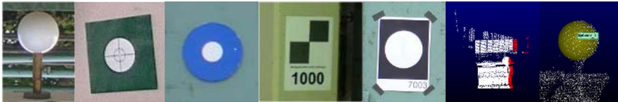
Fig. 2: Targets for semi-automatic registration of scans: Trimble sphere and target, Leica HDS target, paper targets of Z+F and FARO, scan and identification of a Trimble sphere
