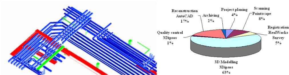
Fig. 7: Selected test area of project 2 for 3D CAD modelling of the pipe line system (left) and expenditure of human labour for the project 2 using Trimble system (right)
