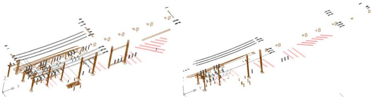
Fig. 6: Comparison of a 3D model (project 1) constructed from HDS3000 data with cyclone (left) and constructed from GS101 data with 3Dipsos (right) in the same elapsed time
