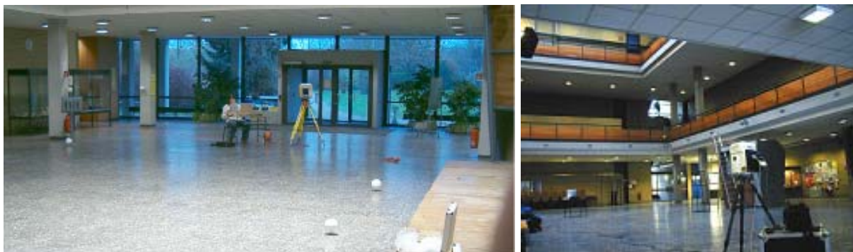
Fig. 2: Terrestrial laser scanner in the 3D test field scanning white spheres.
