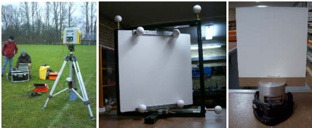
Fig. 6: Trimble GX on a heavy-duty tripod (left), swivelling planar white stone slab (centre) and white colour plate (right).
