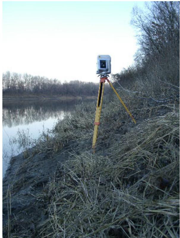
Fig. 15: Scanner in a warped embankment of the river Tisza
