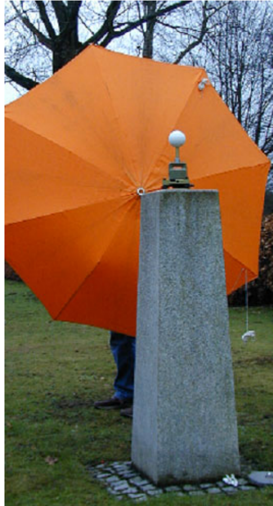
Fig. 10: Background contrast for automatic detection of spheres in the video frame before scanning
