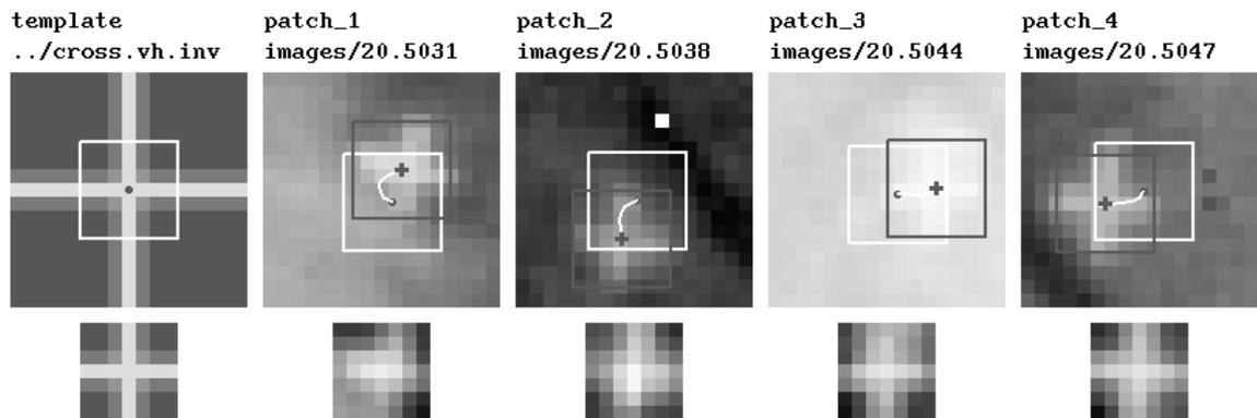
Figure 2a: Template matching of four signalled points (30  $\mu\text{m}$  image data)
