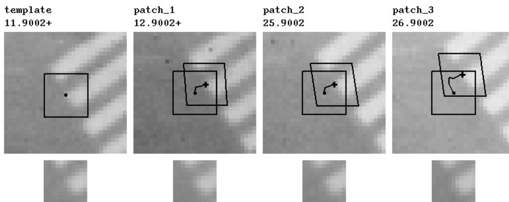
Figure 3: Multiple image matching of four tie points (30  $\mu\text{m}$  image data)
