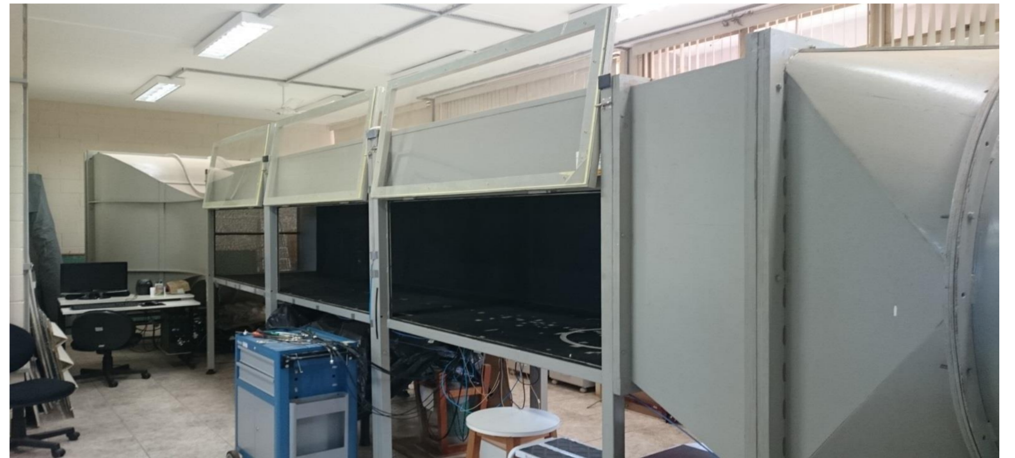
Overview of the wind tunnel in the Laboratory of Environmental Comfort and Applied Physics (LaCAF) in Campinas, Brazil
