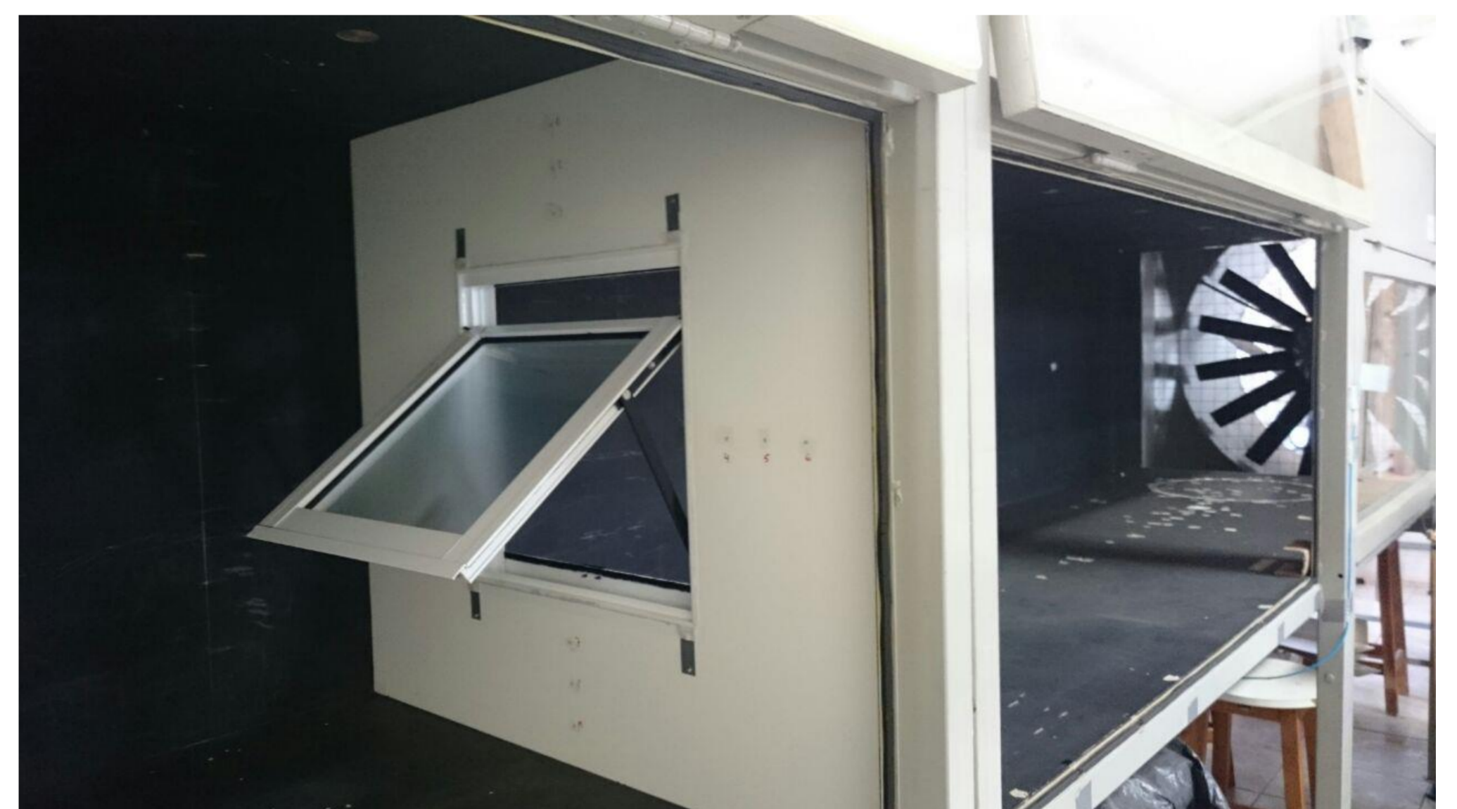
Brazil window installed in the wind tunnel
