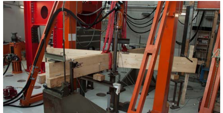
Picture 2: Test setup for the new connection
