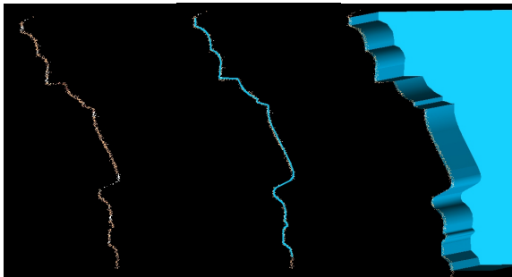
Figure 17: Modelling of ornaments by laser scanning data: cutting of the point cloud (left), CAD line derived from the laser scanning data (centre), extrusion of the CAD line (right).
