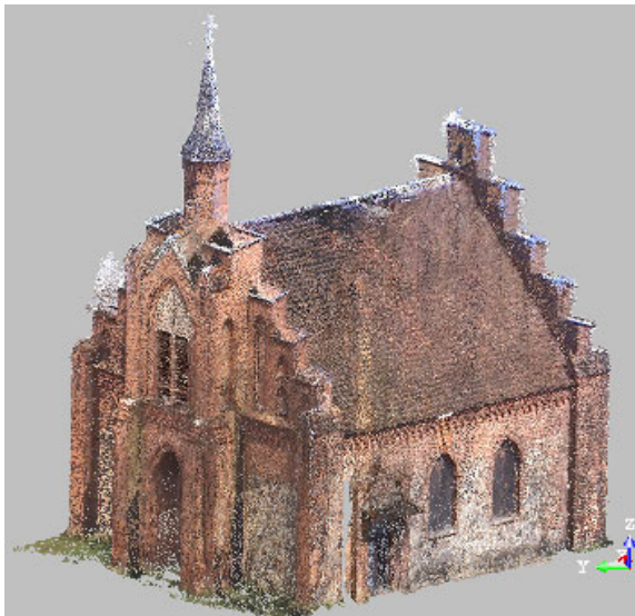
Figure 6: Entire point cloud of church Raduhn represented with RGB values of the point cloud
