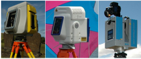
Figure 1: Terrestrial laser scanning systems used: Trimble GX (left), Trimble GS101 (centre) and the IMAGER 5006 from Zoller + Fröhlich (right)
