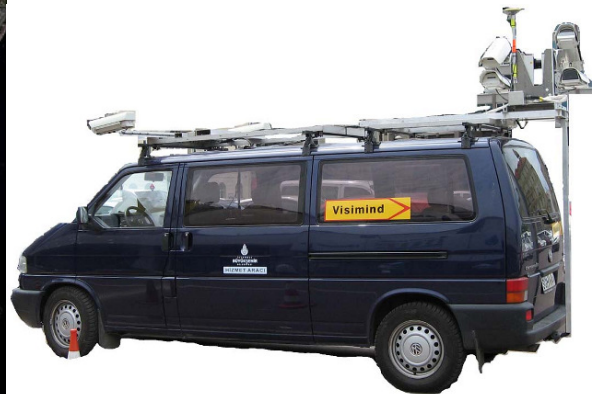
Figure 2. Sensor configuration on the mobile mapping van of VISIMIND AB
