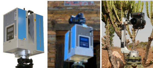
Figure 3: Laser scanner IMAGER 5006 (left), with mounted Nikon D40 camera (centre) and Nikon D200 camera on nodal point adapter
